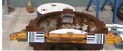
Figure 12: Fiducials and their placement on the crucible (as seen from the PTZ camera).
