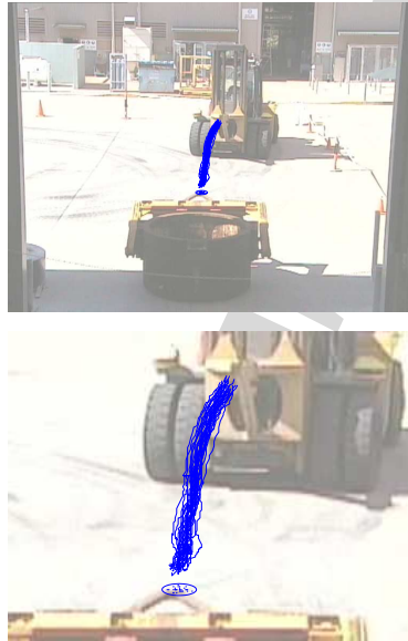
Figure 20: Pick up approach trajectories, superimposition of 29 pickups. The dots and the ellipse around the crucible handle show the variability of the crucible location across this set of manoeuvres. The top figure shows an overview of the experiment area, and the bottom figure shows a close-up on the paths themselves. For reference, the handle width is about 2m and the pick up hole approximately 20cm across.
