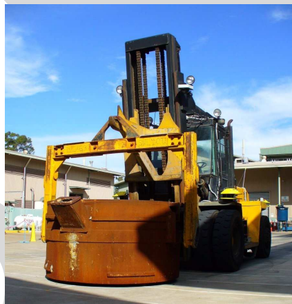
Figure 1: A Hot Metal Carrier in the process of picking up the crucible.
