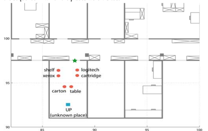
Fig. 16 First ‘unknown’ place at the time of place recognition. The configuration of the objects is different from that of the same place in Fig. 12. Note - The carton is above the table & xerox is above the shelf .
